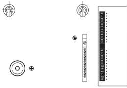
There is a dedicated terminal for the live and neutral of each output circuit. A shared Earth bus bar is mounted on the chassis of the dimmer.
