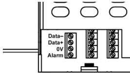
DMX input is connected through a 4-way screw terminal block located on the control PCB.
