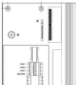
Mains supply will come in from the top of the dimmer, with phases and neutral being wired to the isolator input terminals. Input terminals will accept a maximum 35mm<sup>2</sup> cable.
