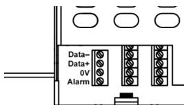
The Alarm Input is connected through a 4-way screw terminal block located on the control PCB (Figure 2-15).
