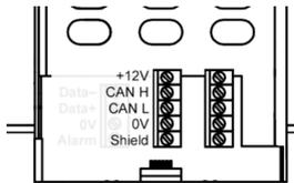
Inside the dimmer, the terminals for network connections use two-part connectors. Pull the connector from the PCB, connect the wires from the CAT 5 cable and push the connector back onto the PCB, ensuring correct orientation.
