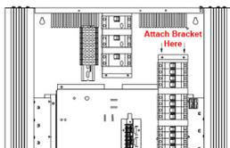
4 . Assemble the metal bracket to the unit in the position shown. Do this by removing the two screws holding the circuit breaker bracket to the enclosure, putting the metal bracket into position and refitting the screws. Once the bracket is in place clip the power supply to the metal bracket such that the N and L terminals are facing to the right.
