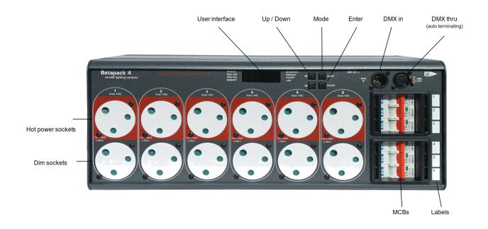
Betapack 4 distributes both dimming and non-dimming ("hot power") to a mixed rig of both tungsten and LED fixtures. Each of the six channels are capable of driving up to 10 amp loads.
