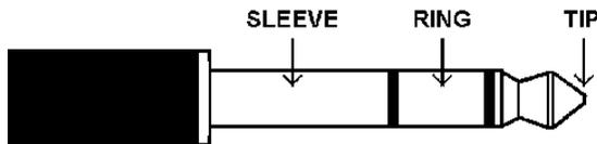
A jack connector provides a remote switch. Short tip to sleeve to simulate a button push.
