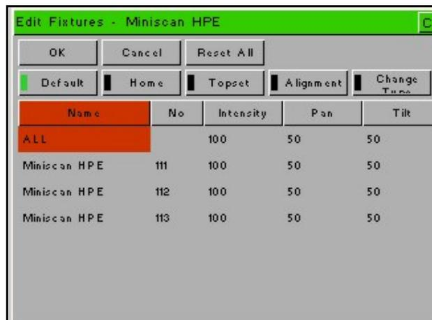
To make changes to a particular fixture or a complete group of fixtures, first select the fixture group. The name of the group is displayed in the header of the window.
