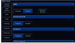
The Universes tab of Setup is a single place for configuring each separate method (“protocol”) of sending lighting data out of the console to your lighting rig.
