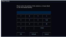
To change a streaming ACN universe's priority, press "Priority" and either enter the new number, or click "Default". Clicking default means this universe will then use the default streaming ACN priority value set in the global streaming ACN settings at the top of the Universes tab of Setup.
