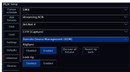
RigSync can be enabled or disabled within the RDM panel of the "Universes" tab within Setup. On FLX, RigSync is disabled by default. On FLX S, RigSync is enabled by default on DMX port 1.
