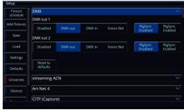
The DMX section of the Universes tab in Setup, allows you to configure the behaviour of the DMX ports of the rear of the console. FLX series consoles have two DMX ports.
