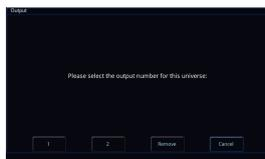
You can then choose which physical output port you wish this Desk Universe to be routed from. FLX series consoles have a pair of DMX outputs on the rear of the console.
