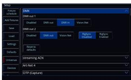
Either of the console's DMX ports, can be configured as a DMX Input rather than an output. Using a male-to-male XLR adapter, this allows you to send a DMX signal into your console from an external DMX source, which can then be used to control fixture intensities, or playback levels.
