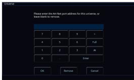
You can choose to send DMX data on any Art-Net 4 universe from 0 to 32,767. It is recommended to avoid using Art-Net universe 0 if you can, and start with Art-Net universe 1, to avoid any offset confusion.
