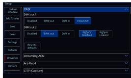
FLX series consoles can receive Vision.Net commands over RS-485, using either of the DMX ports. Once you have chosen the DMX port you wish to receive Vision.Net messages, you can then configure Vision.Net in the Triggers tab of Setup.
