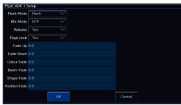
Once you have programmed a channel data UDK, you can configure it. To do this, hold Setup and tap the UDK you wish to configure, to open the UDK Settings.
