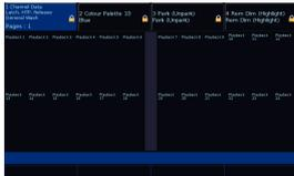
The functionality of the UDKs is displayed in the four boxes, running along the top of the Faders window.
