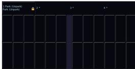
In the Faders window, the normal Park function will be shown, on the onscreen UDK, with the shifted Unpark function shown in (brackets).
