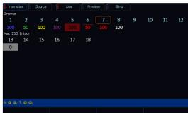
When a fixture is parked, its intensity percentage will be displayed in black in the Output window with a red background, as can be seen for fixture 5 in the image.
