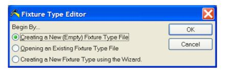
Select "Creating a New (Empty) Fixture Type File" and press OK. A blank fixture file is created (FixTyp1):
