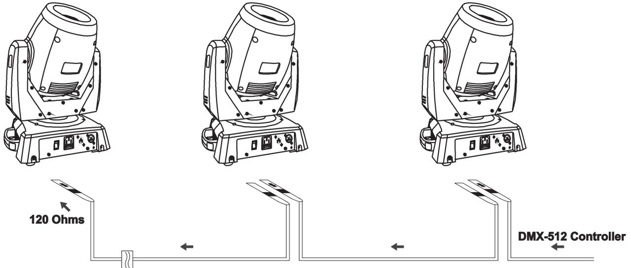
**The wires must not come into contact with each other, otherwise the fixtures will not work at all, or will not work properly.**
